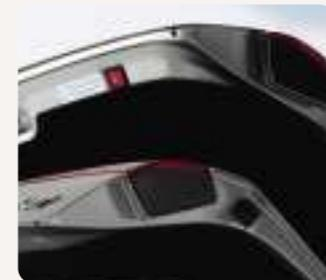
Press the red button in the tailgate and the boot lid closes automatically.
